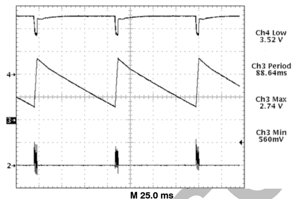
Trace 4– 5.0 V Supply Voltage (2.0 V/div.) Trace 3– Soft Start Timing Capacitor (1.0 V/div.) Trace 2– Inductor Switching Node (2.0 V/div.)
